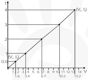
Here, the I – V graph is almost straight. The resistance of the resistor can be calculated as given
