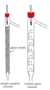
*Fig.*12.7 *Different types of fractionating columns.*
