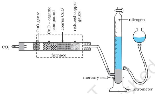
**Fig.12.15** Dumas method. The organic compound yields nitrogen gas on heating it with copper(II) oxide in the presence of  $CO_2$  gas. The mixture of gases is collected over potassium hydroxide solution in which  $CO_2$  is absorbed and volume of nitrogen gas is determined.
