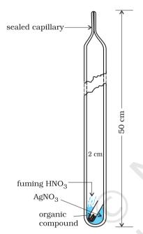
Fig. 12.17 Carius method. Halogen containing organic compound is heated with furning nitric acid in the presence of silver nitrate.
