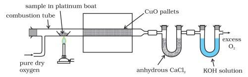
**Fig.12.14** Estimation of carbon and hydrogen. Water and carbon dioxide formed on oxidation of substance are absorbed in anhydrous calcium chloride and potassium hydroxide solutions respectively contained in U tubes.
