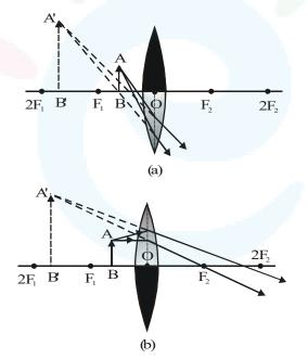
10. An object 5 cm in length is held 25 cm away from a converging lens of focal length 10 cm. Draw the ray diagram and find the position, size and the nature of the image formed.
