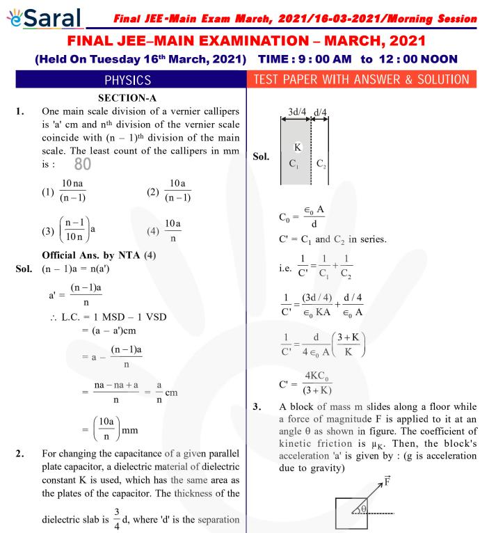
between the plates of parallel plate capacitor. The new capacitance (C') in terms of original capacitance ( $C_0$ ) is given by the following relation :
