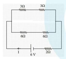
$R_{eq} = \frac{6 \times 12}{6 + 12} + 2$  $= \frac{6 \times 12}{18} + 2$  $R_{eq} = 6\Omega$  $I = \frac{V}{R_{eq}} = \frac{6}{6} = 1 \text{ Amp.}$
