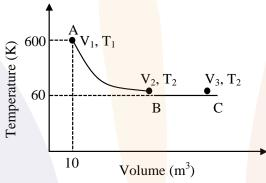
$A \to B$  is an adiabatic process. If the total heat absorbed in the entire process  $(A \to B \text{ and } B \to C)$  is  $RT_2$  ln 10, the value of 2 log  $V_3$  is \_\_\_\_\_.
