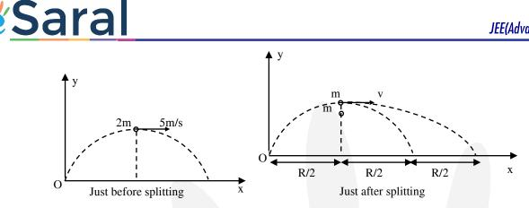
$\therefore$  Time of motion of one part falling vertically downwards is = 0.5 sec =  $\frac{T}{2}$
