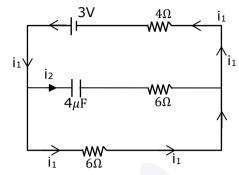
In steady state, no current will pass through capacitor hence capacitor will act as open circuit.  $i_2 = 0$
