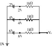
By nodal analysis  $\frac{V_0-2}{1k\Omega} + \frac{V_0-4}{1k\Omega} + \frac{V_0-6}{1k\Omega} = 0$
