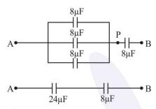
Finally equivalent capacitance
