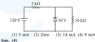
Assuming zener diode doesnot undergo breakdown, current in circuit =  $\frac{120}{15000} = 8 \text{ mA}$  $\therefore$  Voltage drop across diode = 80 V > 50 V. The diode undergo breakdown.
