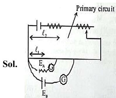
Keeping the primary circuit fixed, if different cells are connected in secondary circuit then emf of the cell is given by
