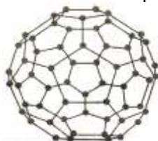
The soccer ball structure of Buckminster Fullerene ( C_{60} )
