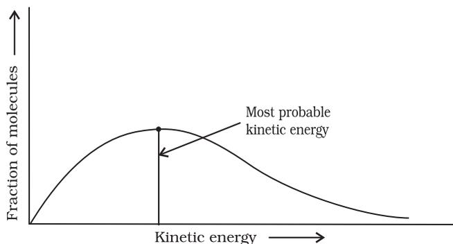
**Fig. 4.8:** Distribution curve showing energies among gaseous molecules
