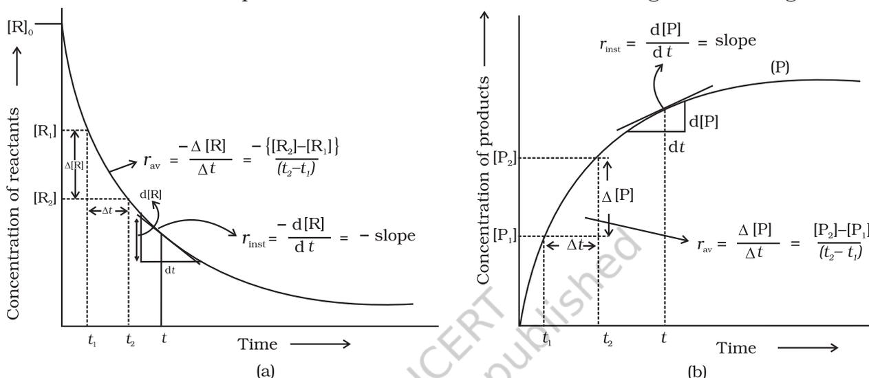
**Fig. 4.1:** Instantaneous and average rate of a reaction
