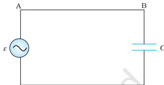
FIGURE 7.8 An ac source connected to a capacitor.
