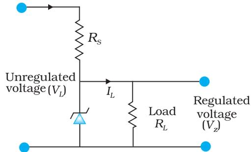
**FIGURE 14.22** Zener diode as DC voltage regulator
