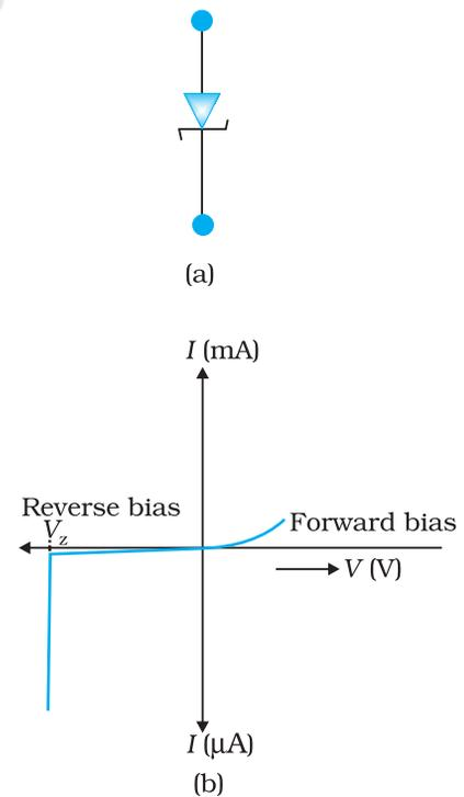
**FIGURE 14.21** Zener diode, (a) symbol, (b) I-V characteristics.
