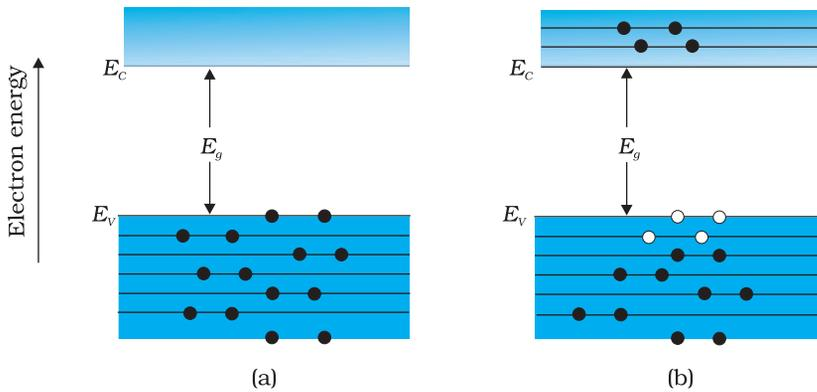
**FIGURE 14.6** (a) An intrinsic semiconductor at  $T = 0$  K behaves like insulator. (b) At  $T > 0$  K, four thermally generated electron-hole pairs. The filled circles (•) represent electrons and empty circles (○) represent holes.
