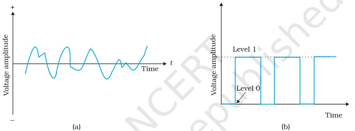
**FIGURE 14.27** (a) Analog signal, (b) Digital signal.
