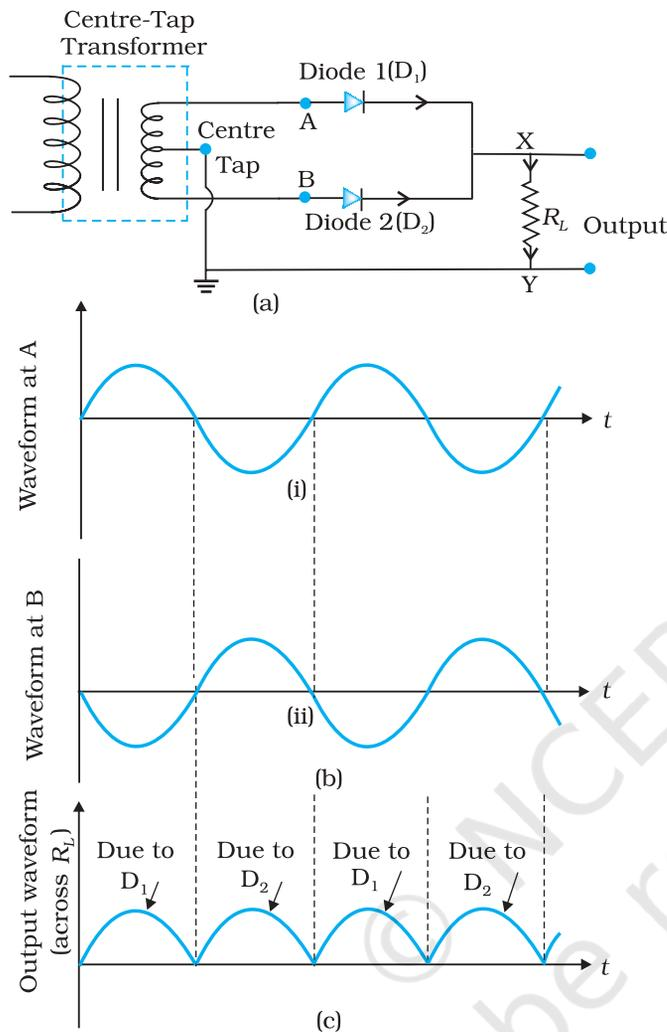
**FIGURE 14.19** (a) A Full-wave rectifier circuit; (b) Input wave forms given to the diode  $D_1$  at A and to the diode  $D_2$  at B; (c) Output waveform across the load  $R_L$  connected in the full-wave rectifier circuit.
