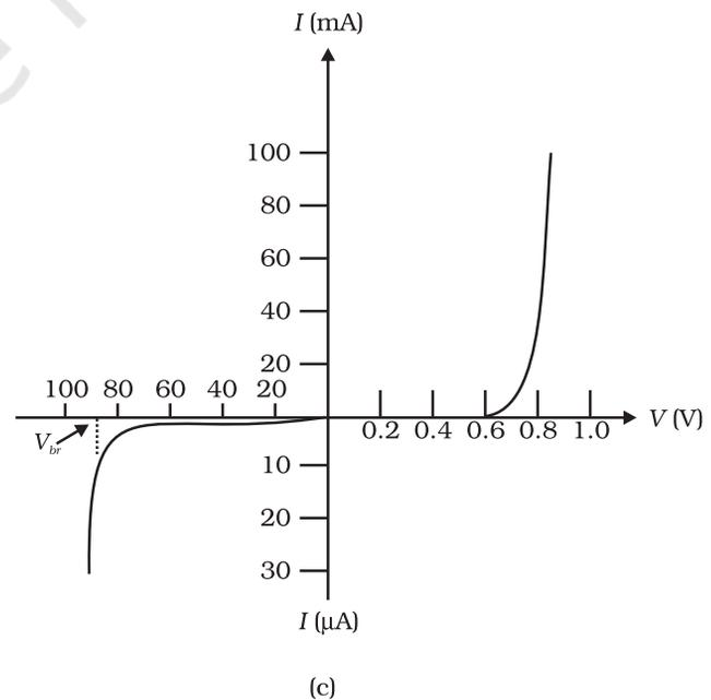
**FIGURE 14.16** Experimental circuit arrangement for studying  $V$ - $I$  characteristics of a p-n junction diode (a) in forward bias, (b) in reverse bias. (c) Typical  $V$ - $I$  characteristics of a silicon diode.
