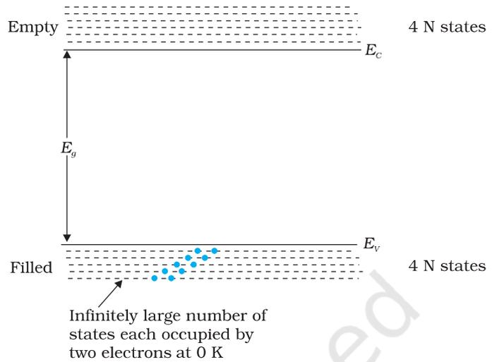
**FIGURE 14.1** The energy band positions in a semiconductor at 0 K. The upper band, called the conduction band, consists of infinitely large number of closely spaced energy states. The lower band, called the valence band, consists of closely spaced completely filled energy states.
