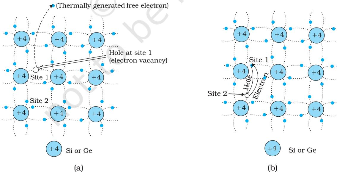
**FIGURE 14.5** (a) Schematic model of generation of hole at site 1 and conduction electron due to thermal energy at moderate temperatures. (b) Simplified representation of possible thermal motion of a hole. The electron from the lower left hand covalent bond (site 2) goes to the earlier hole site 1, leaving a hole at its site indicating an apparent movement of the hole from site 1 to site 2.
