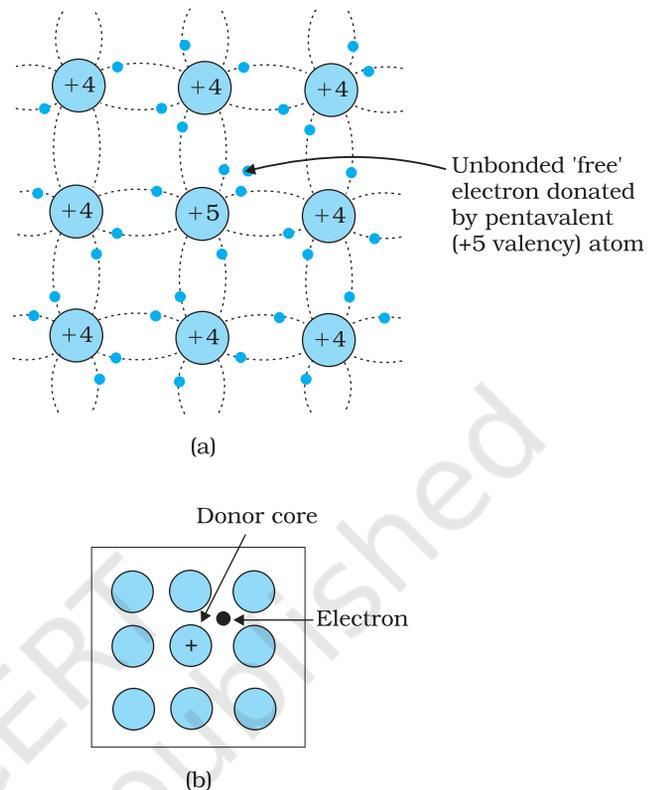
**FIGURE 14.7** (a) Pentavalent donor atom (As, Sb, P, etc.) doped for tetraivalent Si or Ge giving *n*-type semiconductor, and (b) Commonly used schematic representation of *n*-type material which shows only the fixed cores of the substituent donors with one additional effective positive charge and its associated extra electron.
